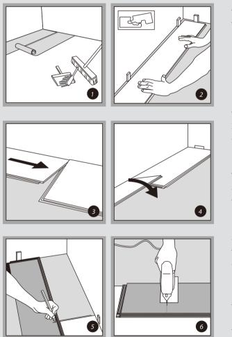
The sub-surface must be absolutely even, dry, clean and stable **[1]**. The installation of a minimum 2mm thick underlay (with moisture barrier for concrete is required). Never overlap edges of the underlay. Tape underlay edges with appropriate adhesive tape. Underlay thicker than 3mm is not advised, except for a solid/firm underlay like Cork for example.
